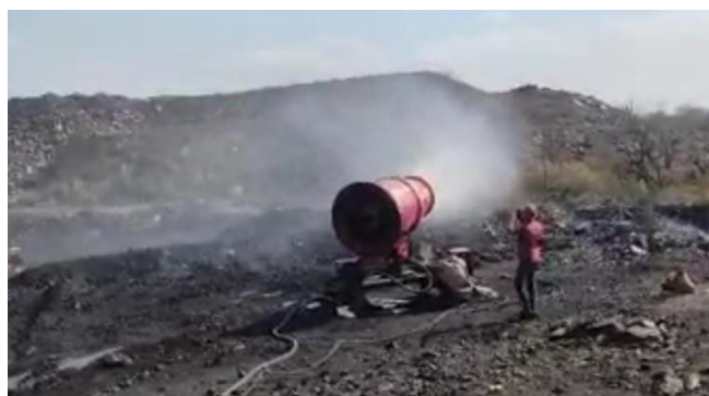
(Water Sprinkling from Trolly Mounted Fog Canon in PB area)
