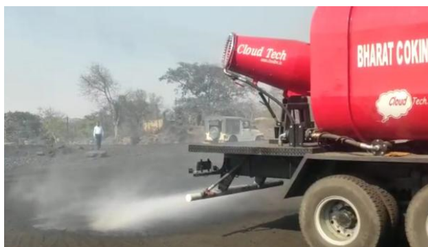
(Water Sprinkling from Truck Mounted Fog Canon)
